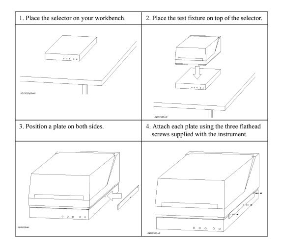
The following steps apply when using two selectors:
