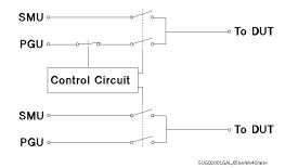
The CH 1 and CH 3 circuits are different from the CH 2 and CH 4 circuits. Each channel has one mechanical relay for SMU and one mechanical relay for PGU, but the CH 1 and CH 3 circuits also have a semiconductor relay for PGU. The relays are controlled by the 4155/4156 via the control circuit.
