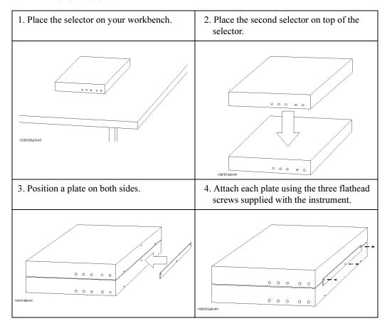
Attach the selector to the shielding box as shown below:
