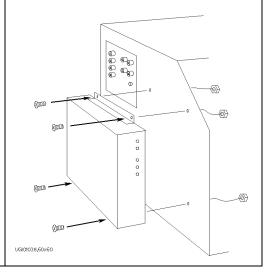
If you use the 16441A R-box, attach the R-Box to the selector on the shielding box as shown below:
