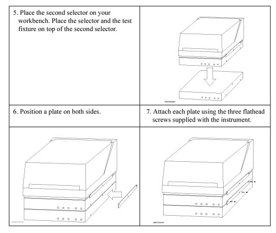
If you use the 16441A R-box, attach the R-Box to the selector as shown below:
